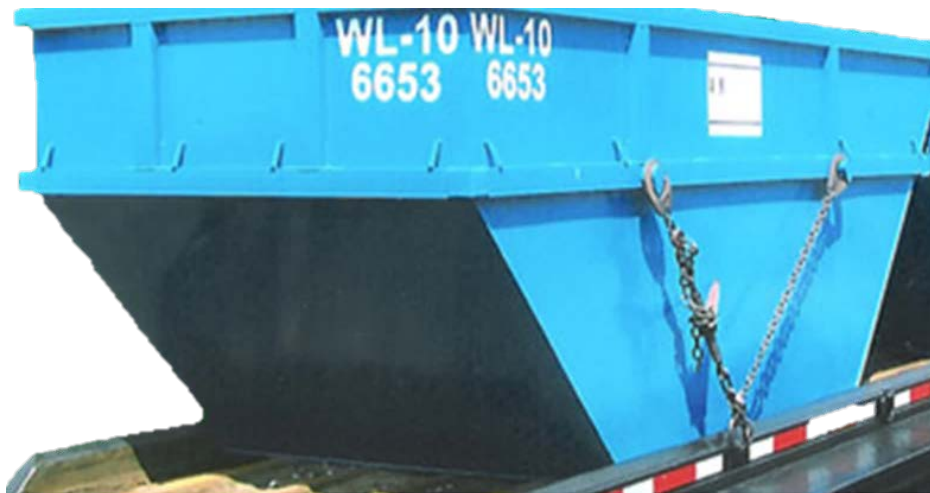
Example: Tiedowns secured to the sides on both sides
