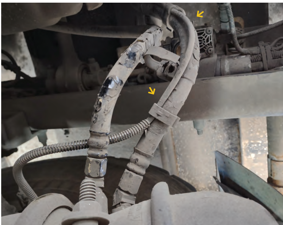
Picture 2. Showing crossed lines. The supply line is going to the modulator valve. This is wrong. Also, the condition of the chamber and hose indicates this condition has existed for quite a while.
