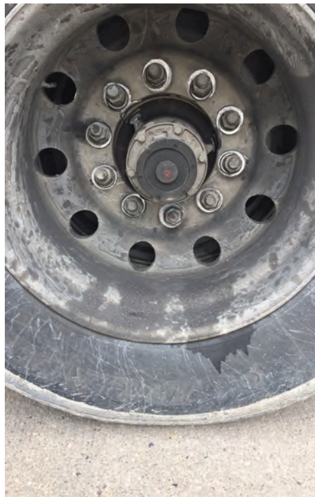
Submitted by Cpl. Denisuk: The wheel was visibly wobbling as the truck drove in for inspection - loose wheel fasteners.
