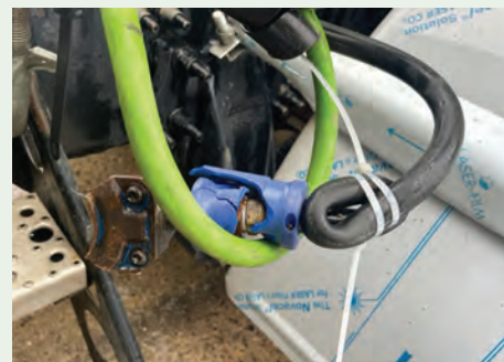
Submitted by Cpl. Finnen: When this unit came over the scale, the officer noticed the service glad hand was not attached and was broken. The hose was crimped, not allowing airflow when brakes were applied. The trailer also had no operational service brakes. The driver was told by his boss to bring the truck from Dryden, Ontario, to Winnipeg, Manitoba, for repairs.
