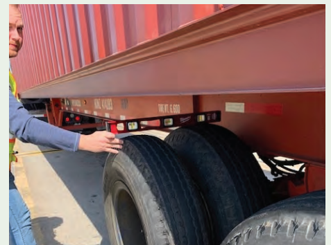
Tire Anomaly Detected - Tire height difference issue.
