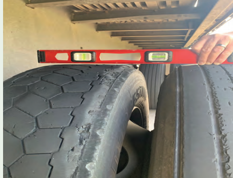
Tire Anomaly Detected - Tire with height difference and cupping.
