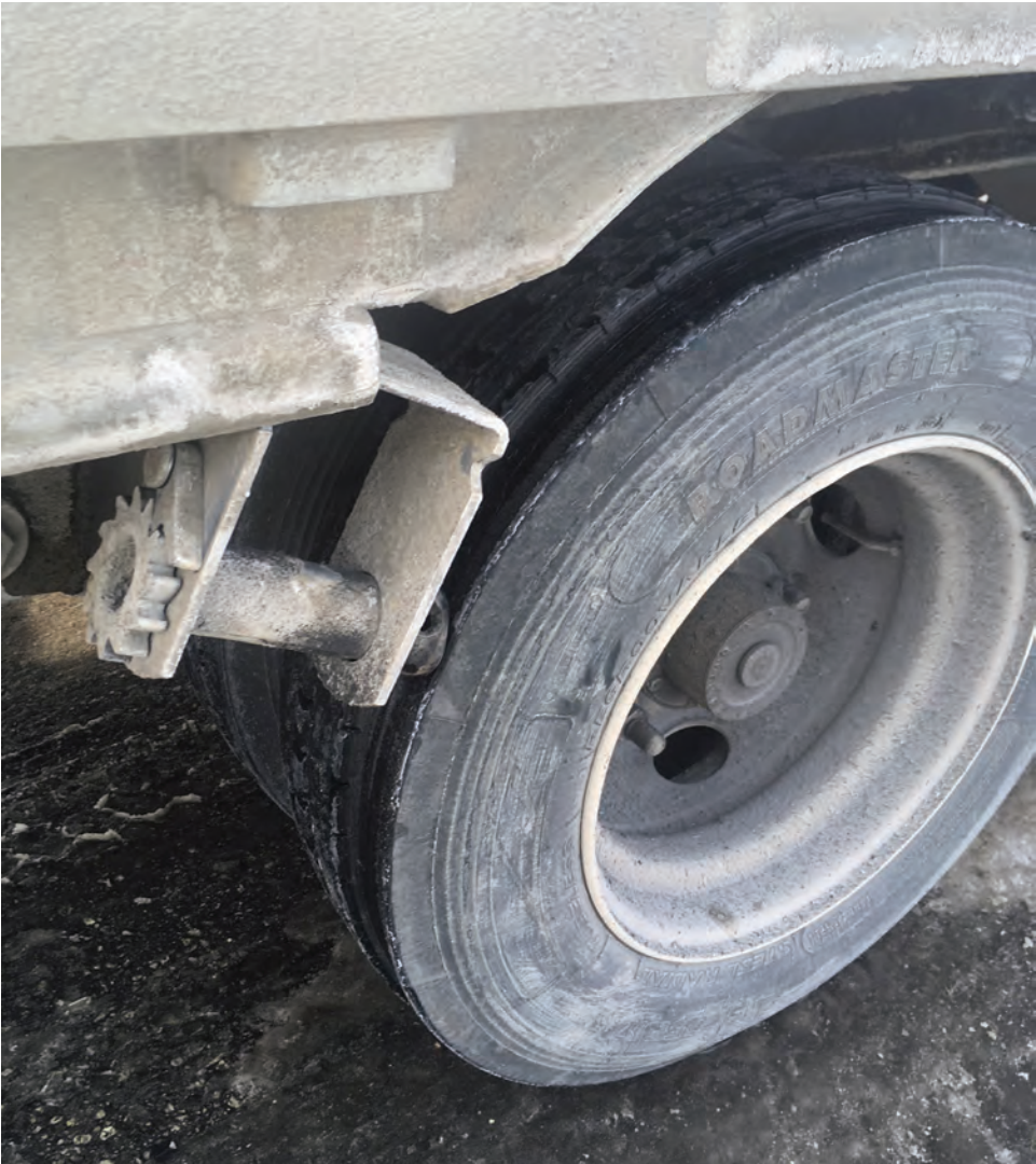
Submitted by Cpl. Finnen: The driver was new to his company and had just picked up the trailer. There was no stop in place for the cargo securement device and it had slid back and rubbed a large indent in the tire.
