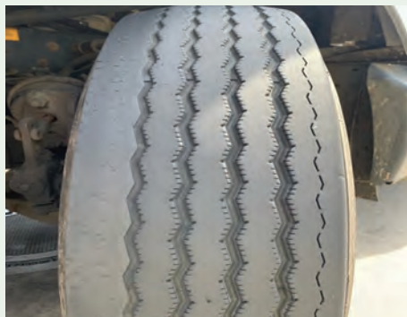
Tire Anomaly Detected - Inside tire worn.
