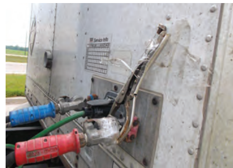
Submitted by Cpl. Williment: This "repair" of a leaking air hose was found on a vehicle reporting to scale.
