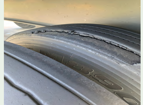
Tire Anomaly Detected – Partial tread separation, this is documented as a violation but is not an out-of-service condition.
