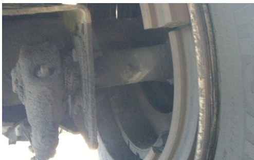
Broken Drum. OOSC, Part II, g.(4) / 393.47(a)-U.S.
