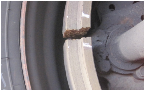
Broken Drum. OOSC, Part II, g.(1) / 393.47(a)-U.S.
