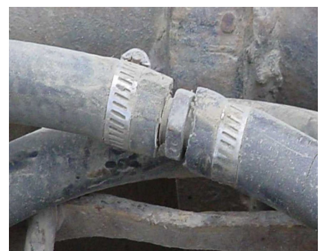
This improper brake hose repair is an out-of-service violation.
