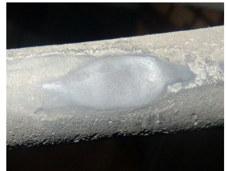
A reduction in brake hose diameter (e.g. due to active chafing) is a violation.
