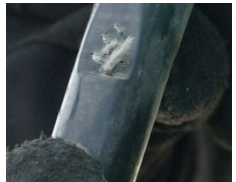
A brake hose chafed into the reinforcement ply is an out of service violation.
